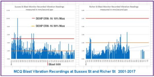
Figure 1 MCQ Blast Vibration monitoring 2001-2017 at End-Sussex & 58-Richer
